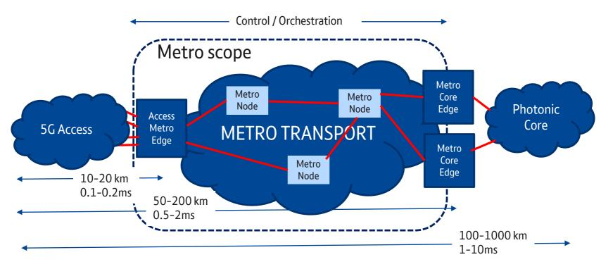
Access Metro Edge Node (AMEN) – multiple ubiquitous access technologies, cloud enabled (storage, compute) Metro Transport Network – metro node: pure transport
