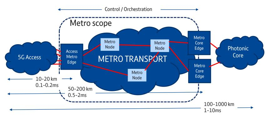
Access Metro Edge Node (AMEN) – multiple ubiquitous access technologies, cloud enabled (storage, compute) Metro Transport Network – metro node: pure transport Metro Core Edge Node (MCEN) – Larger cloud capabilities
